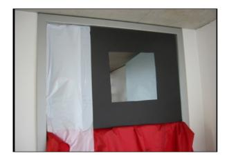
Alternatively, use a Verification Plate in an optional double hole Door Panel, or use the optional Flex Duct with a 400 sq. in. hole in a plate on the end.
