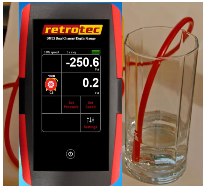
Figure 71: The gauge displaying a negative pressure (-250.6 Pa).
