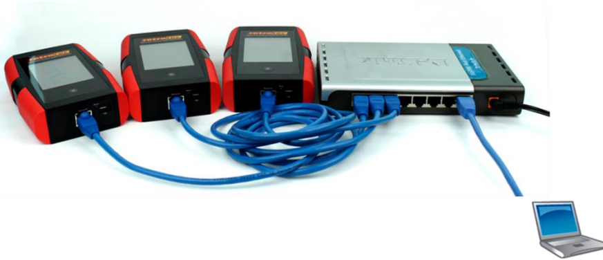
Figure 56: Connect multiple gauges to a wired network using a powered Ethernet Switch
