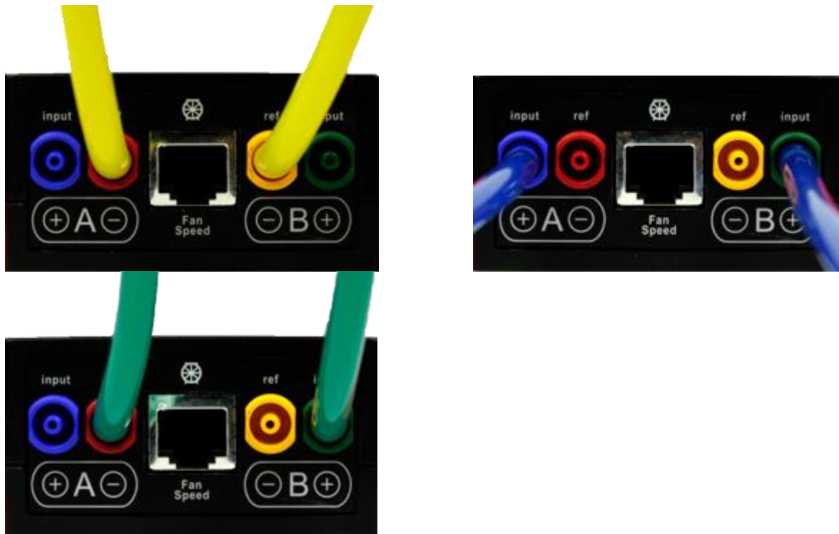
Figure 63: Yellow tube between Channel A & B. Blue tube check of positive ports. Green from negative to positive ports.
