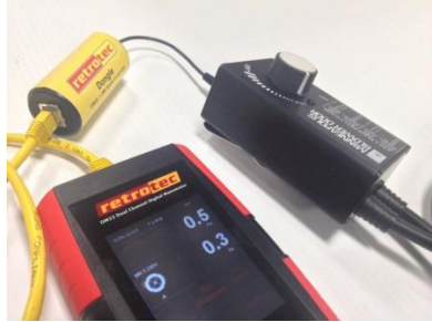
Figure 12: Control a TEC fan using the gauge and TEC Fan Speed Control Adapter (produced by Retrotec)
