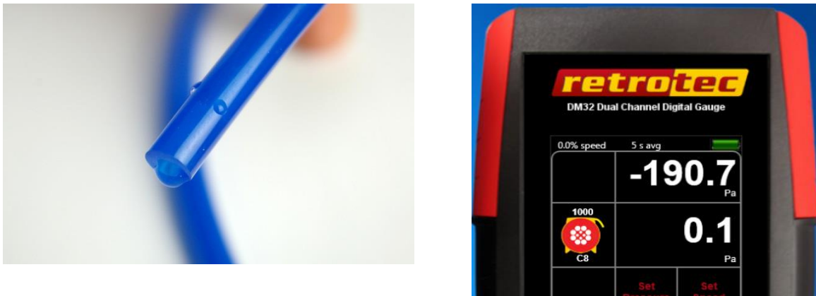
Figure 68: Water in the reference tube (left); high fixed pressure due to water (right).
