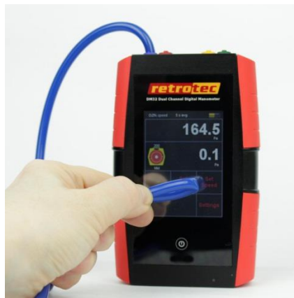
Figure 67: Errors in pressure reading from a pinched tube.
