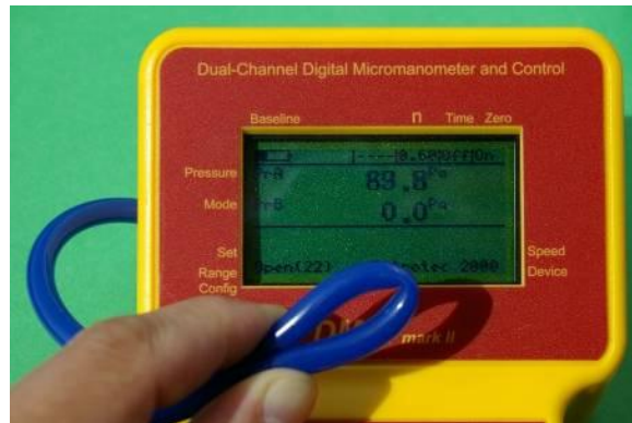
Figure 15: Errors in pressure reading from a pinched tube.
