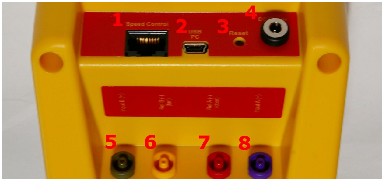
Figure 1: DM-2 back panel with pressure ports and electrical connections
