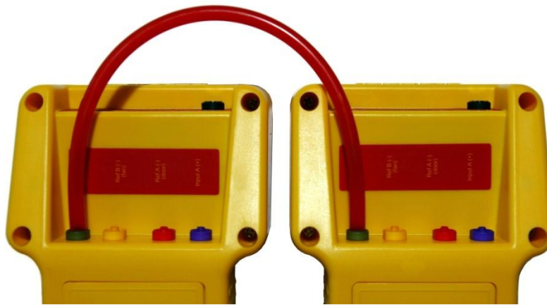
Figure 8: Gauge field check configuration: Cross gauge check
