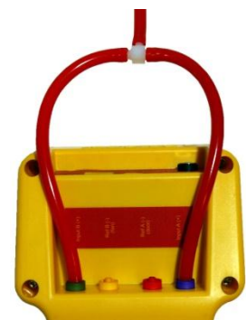
Figure 9: Fan Pressure check using a T-connection
