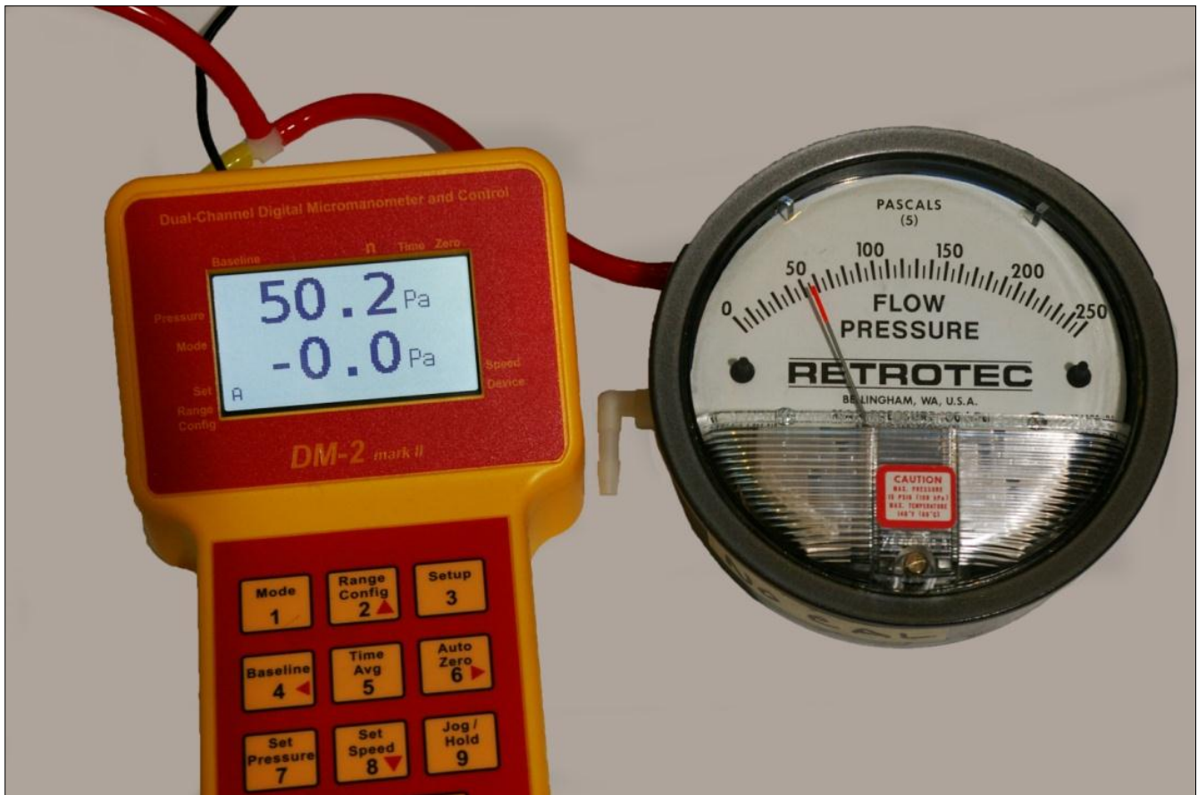
Figure 5: Digital and analog gauges display a pressure of 50.2 Pa. (RetrotecDigital DM-2 left); Retrotec's magnehelic gauge system (right).
