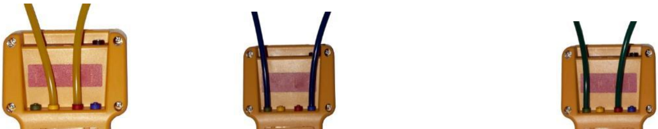
Figure 6: Yellow tube between Channel A & B. Blue tube check of positive ports. Green from negative to positive ports.
