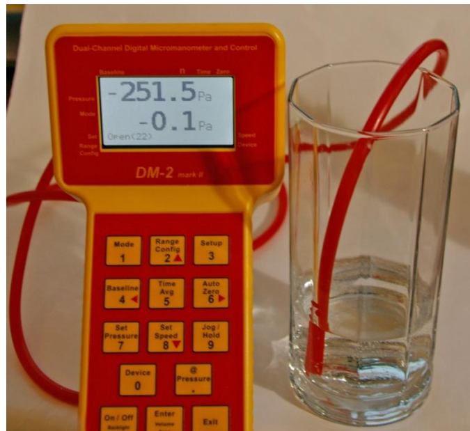
Figure 4: The gauge displaying a negative pressure (-251.5 Pa).
