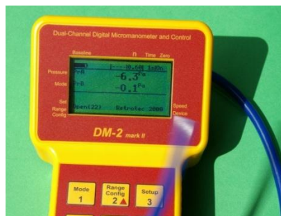
Figure 13: The effect of a moving tube on pressure readings.
